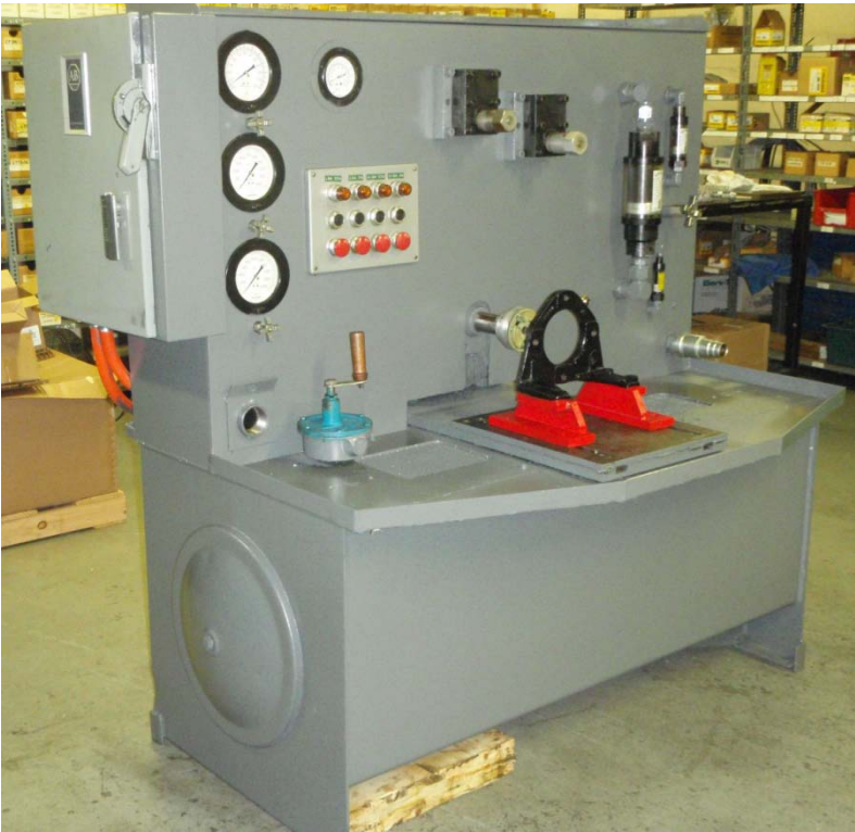
Pump Test Bench:
